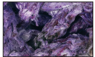
Excessive Internal Abrasion
