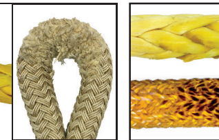
Heat Damage - Melting/Charring
